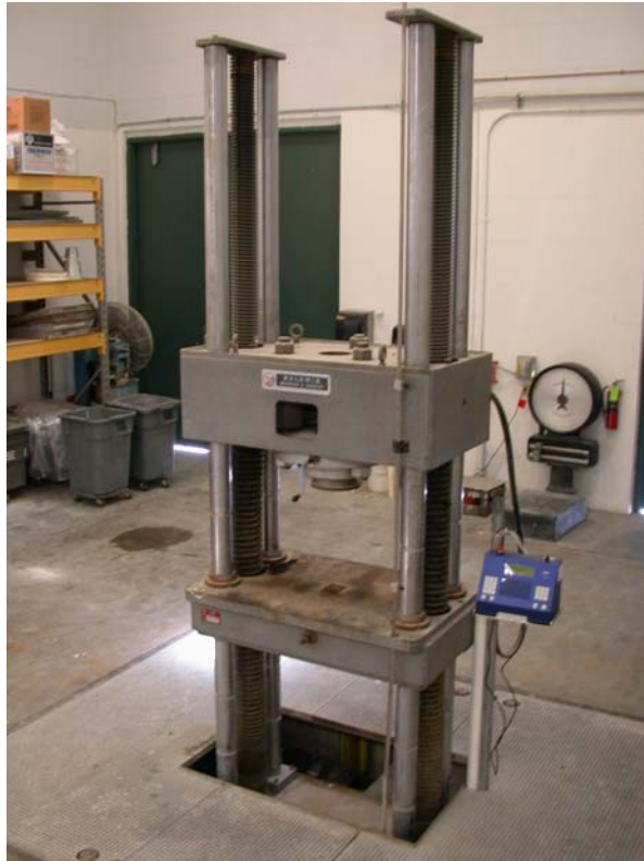
Baldwin 200K universal test frame with ADMET digital retrofit (blue unit on post at right).
